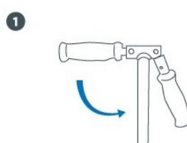
Press the locking buttons to remove the handlebars from the steering column.
