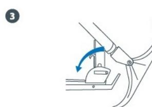
Loosen the clamp of folding mechanism. Pull up the plastic lever. Set the steering column into the level position.
