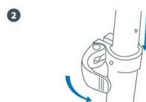
Open the quick release clamp and press the locking button. Slide the steering column to the full-down position.
