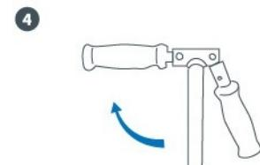
Insert the handlebars into the holes in the steering column. The locking buttons will automatically secure the handlebars when reaching the desired position.
