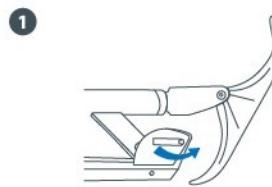
Loosen the clamp of folding mechanism.
