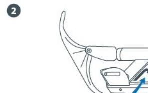
Pull the plastic lever and set the steering column in the upright position. Lock the clamp.
